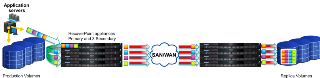
Figure 1. Distributed consistency group architecture
